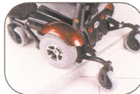
Patented obstacle climb suspension on front castor
